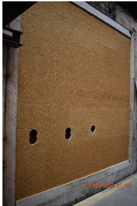
Photo No. 4 Holes drilled for insulating construction
