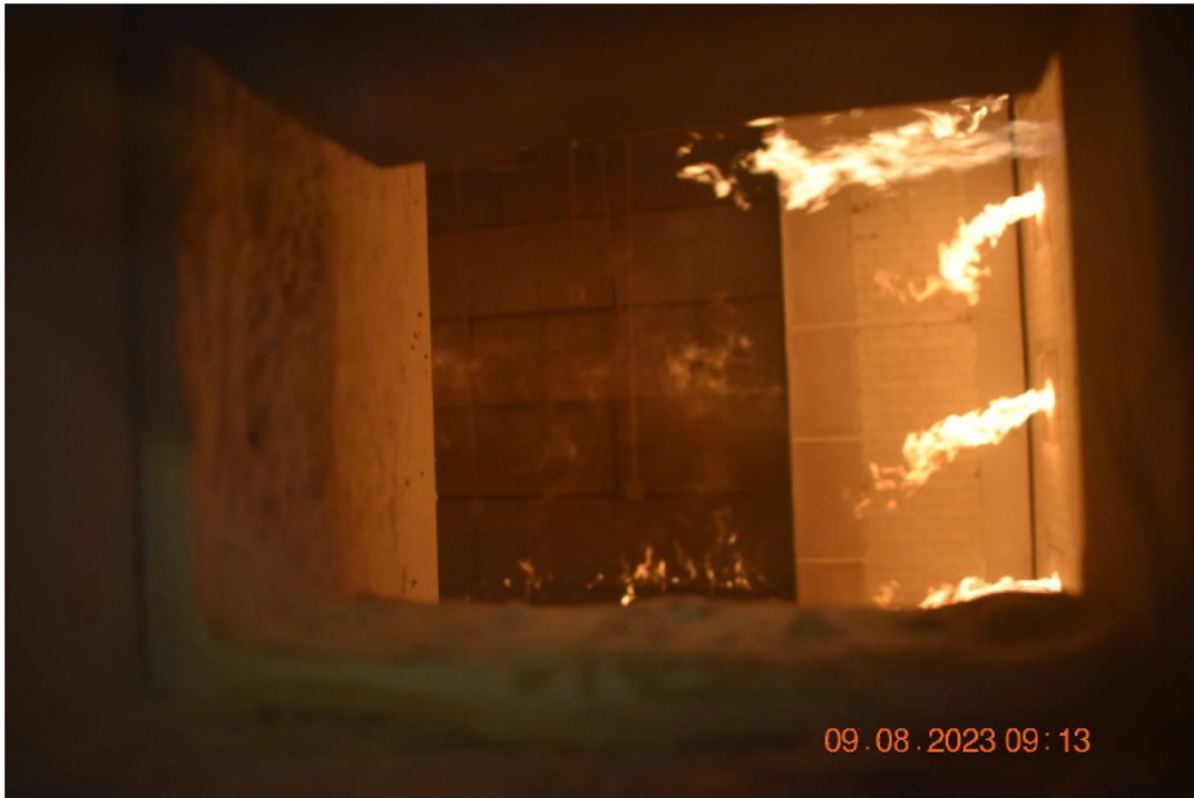
Photo No. 13 Test specimen seen from exposed side 11 minutes into the test
