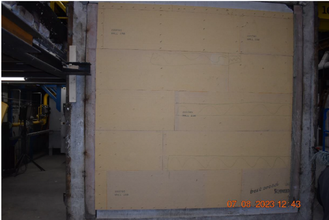
Photo No. 9 Outer layer of wood fiber board seen from unexposed side
