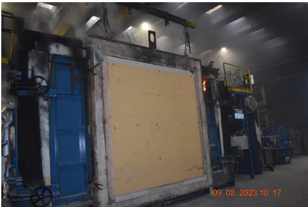
Photo No. 18 Test specimen seen from unexposed side 75 minutes into the test
