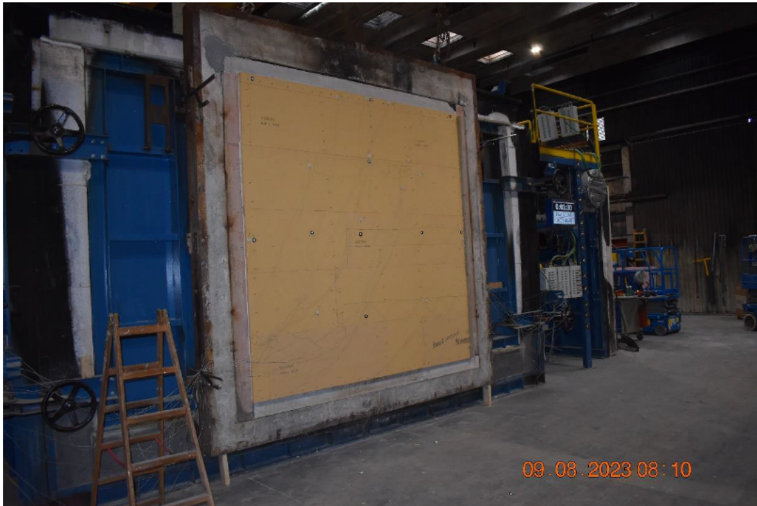
Photo No. 11 Test specimen seen from unexposed side before test start
