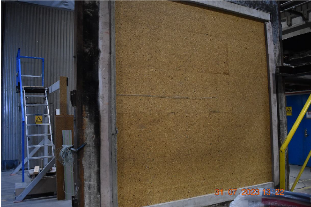
Photo No. 3 Inner layer of boards seen from exposed side
