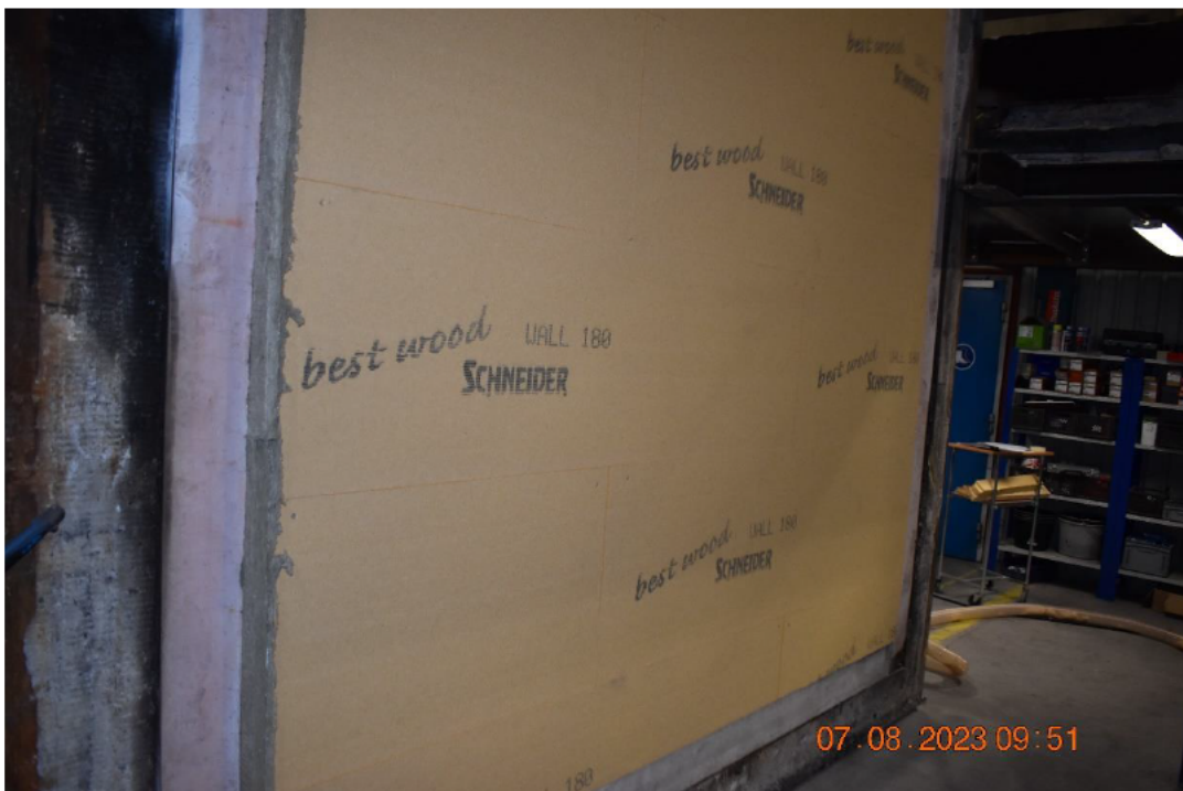
Photo No. 6 Outer layer of wood fiber board seen from exposed side
