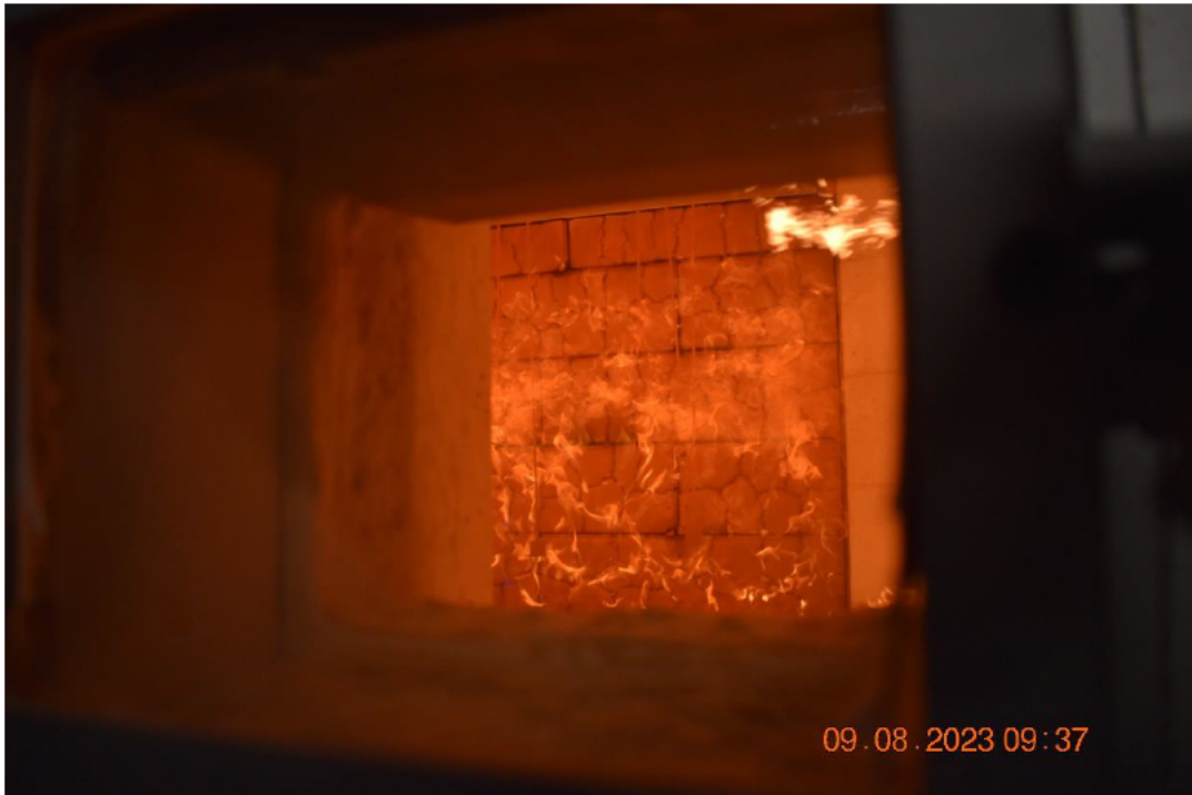
Photo No. 15 Test specimen seen from exposed side 35 minutes into the test
