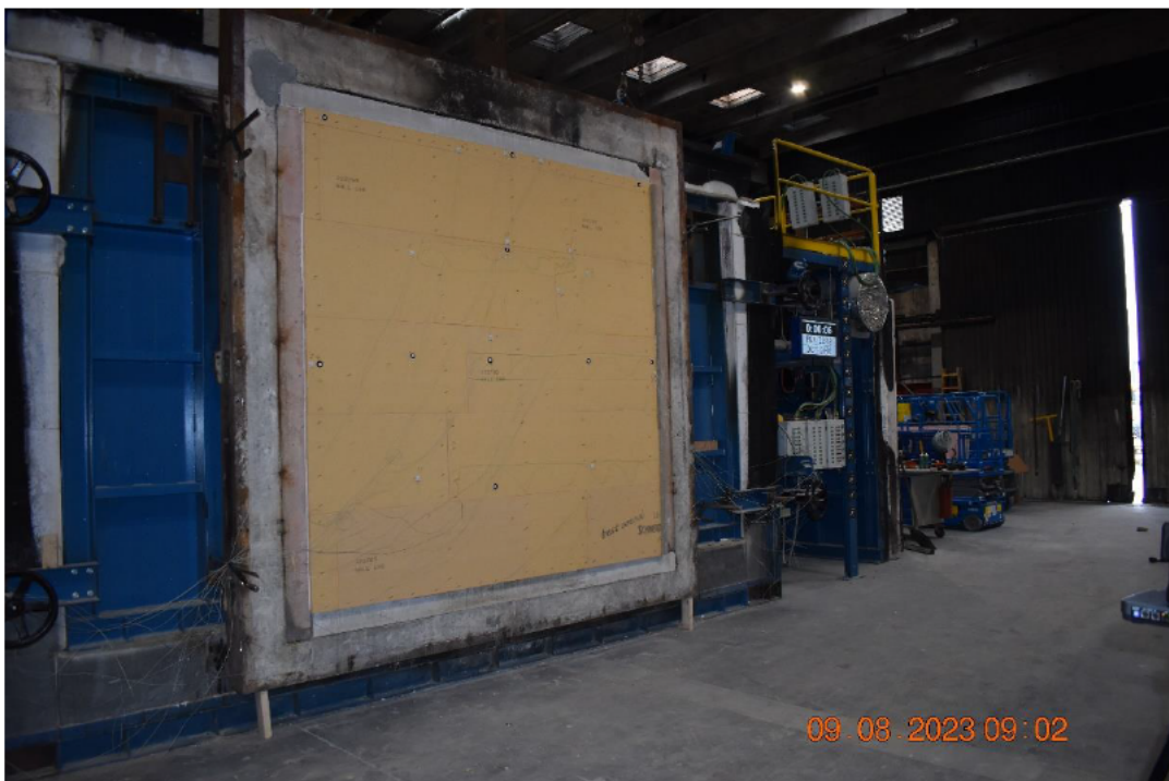
Photo No. 12 Test specimen seen from unexposed side at test start
