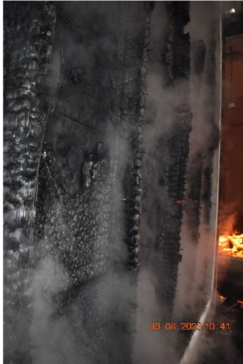
Photo No. 19 Test specimen seen from exposed side after the test
