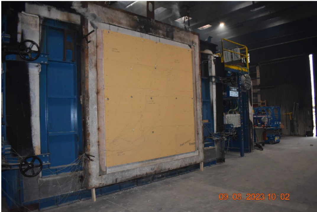
Photo No. 17 Test specimen seen from unexposed side 60 minutes into the test
