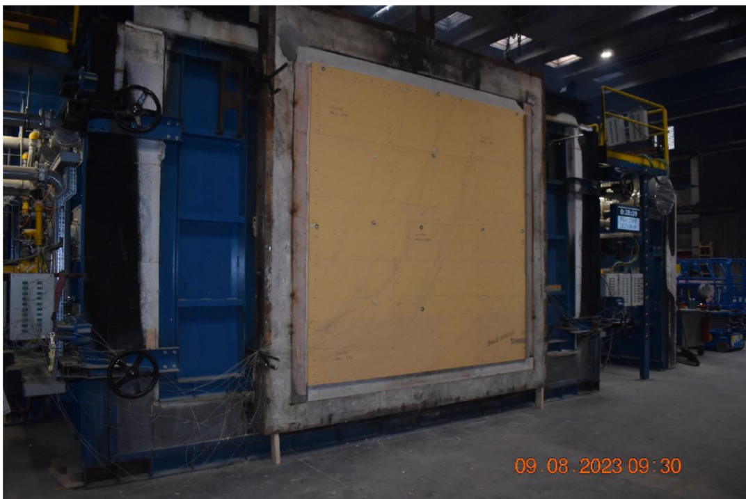
Photo No. 14 Test specimen seen from unexposed side 28 minutes into the test
