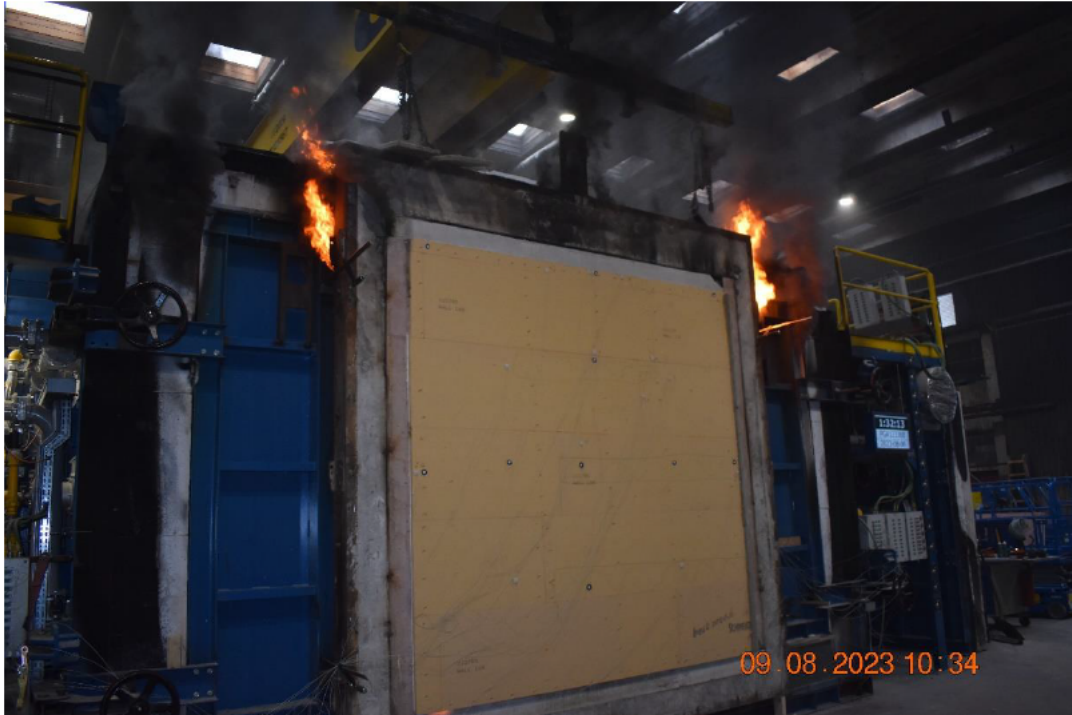
Photo No. 19 Test specimen seen from unexposed side at test end
