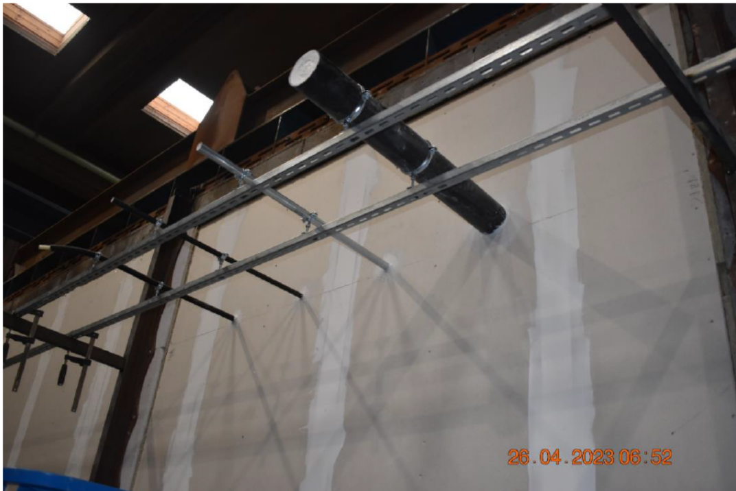
Photo No. 4 Test specimen seen from unexposed side during mounting
