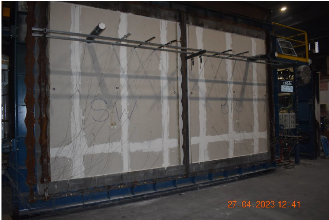
Photo No. 15 Test specimen seen from unexposed side after 60 minutes of testing
