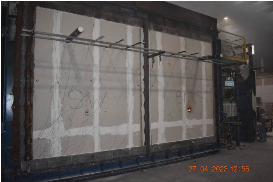
Photo No. 17 Test specimen seen from unexposed side after 75 minutes of testing
