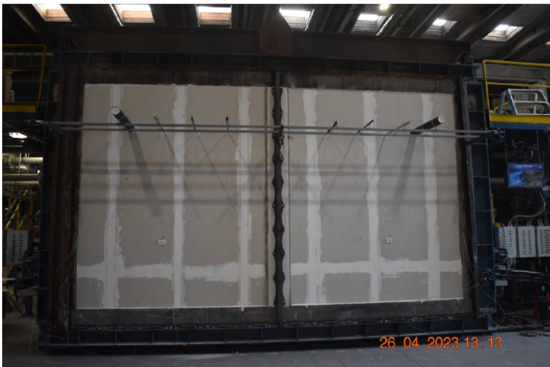
Photo No. 6 Test specimen seen from unexposed side before test start
