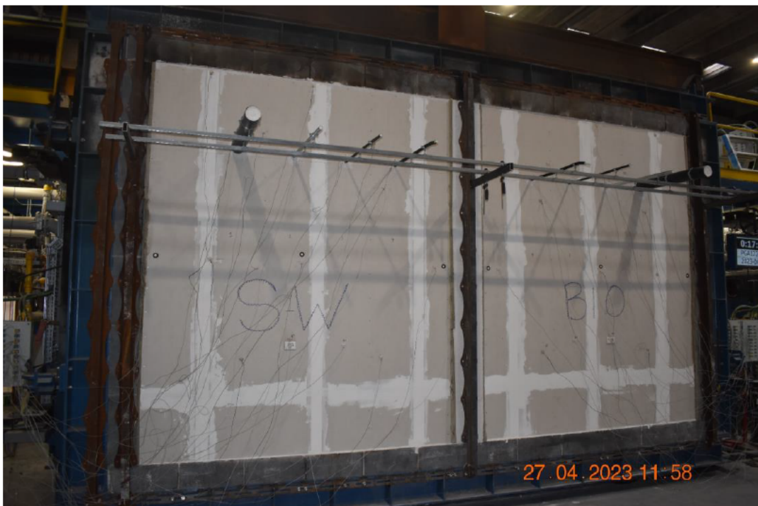
Photo No. 12 Test specimen seen from unexposed side after 17 minutes of testing
