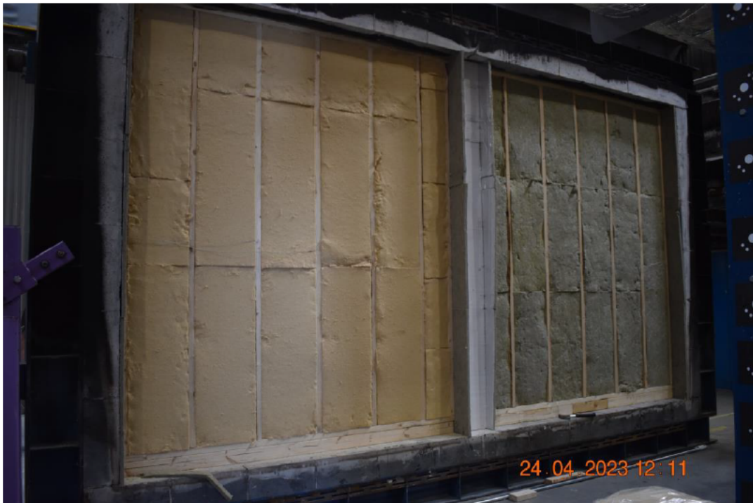
Photo No. 2 Supporting construction seen from exposed side during mounting
