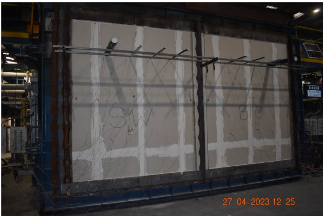
Photo No. 14 Test specimen seen from unexposed side after 45 minutes of testing
