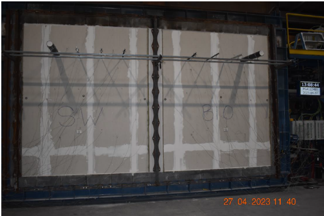
Photo No. 10 Test specimen seen from unexposed side before test start
