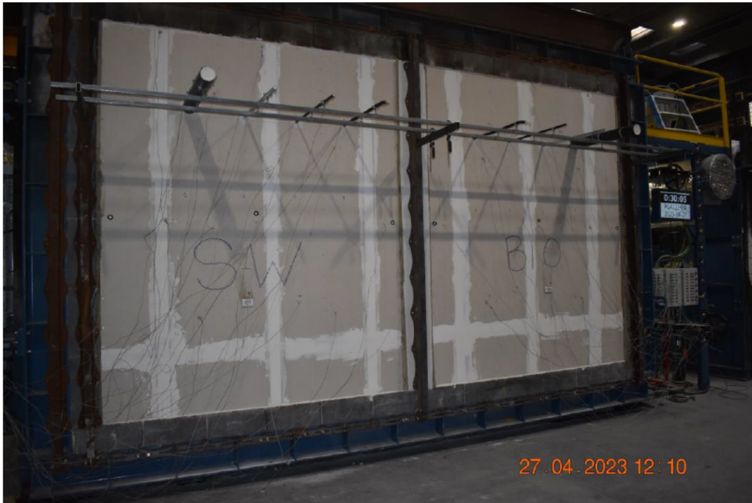
Photo No. 13 Test specimen seen from unexposed side after 30 minutes of testing
