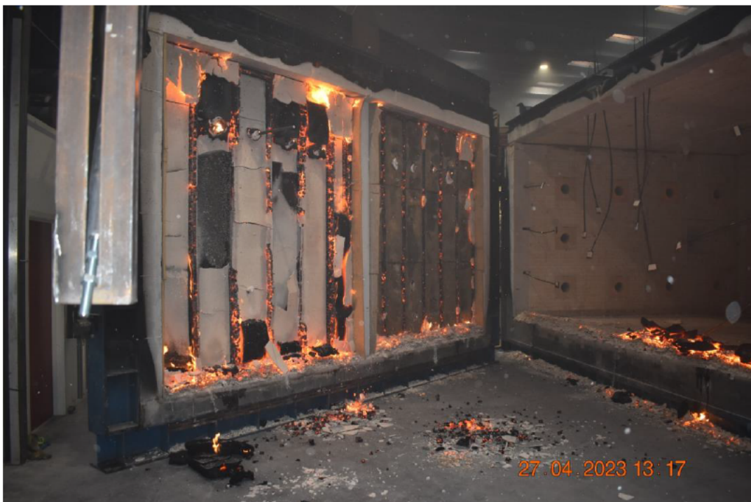
Photo No. 20 Test specimen seen from exposed side after the test
