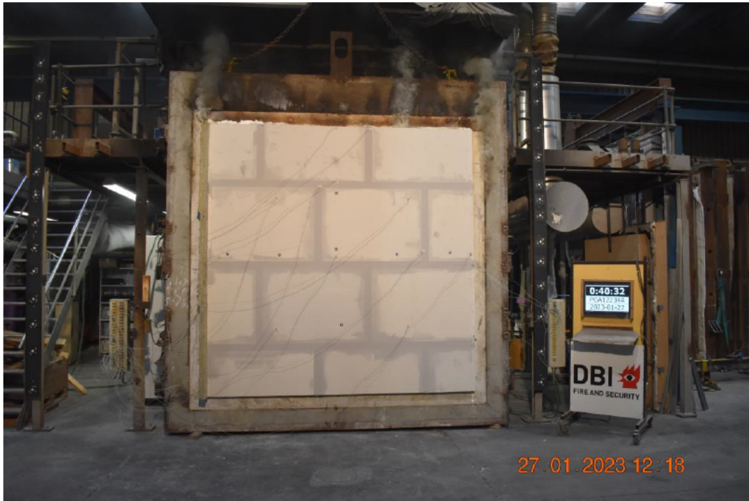
Photo No. 13 Test specimen seen from unexposed side 40 minutes into the test
