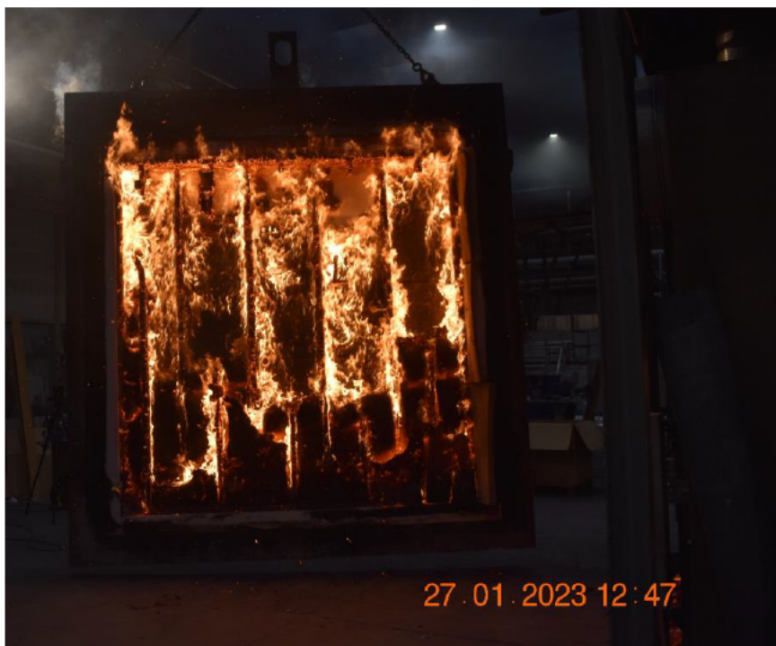
Photo No. 16 Test specimen seen from exposed side after the test
