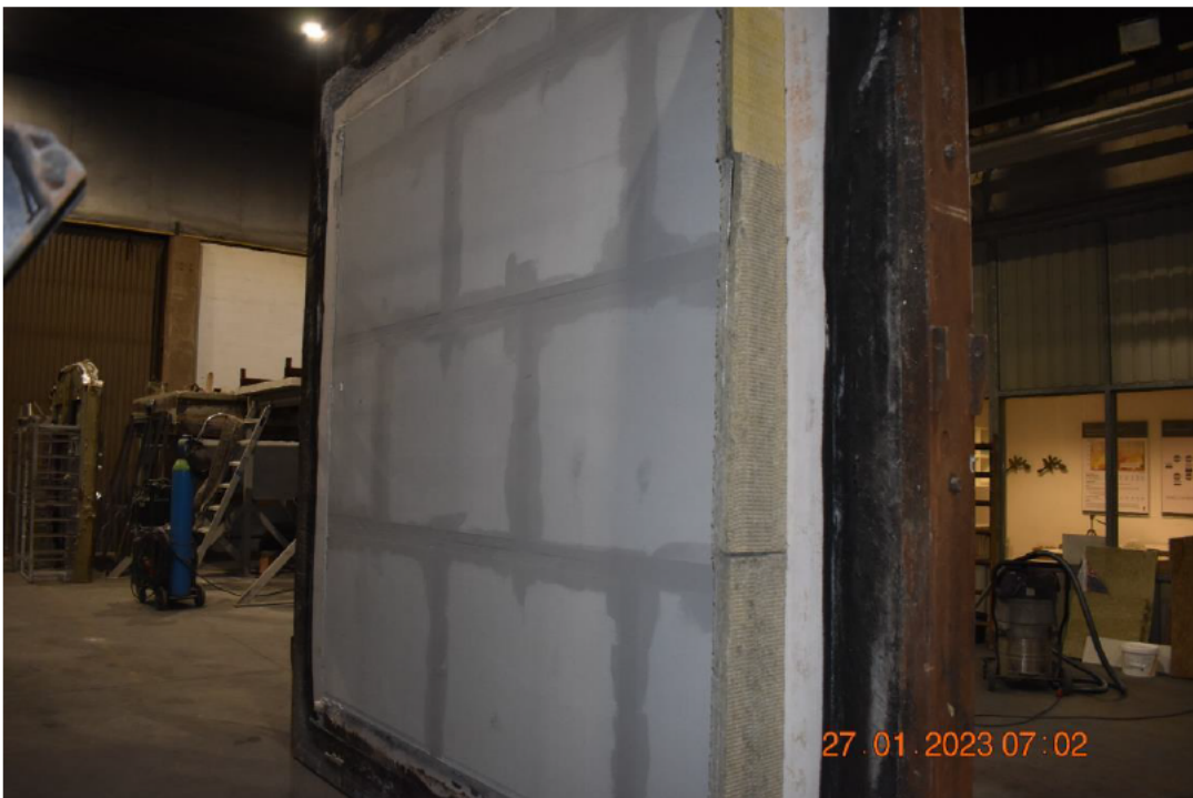
Photo No. 6 Test specimen seen from exposed side during mounting
