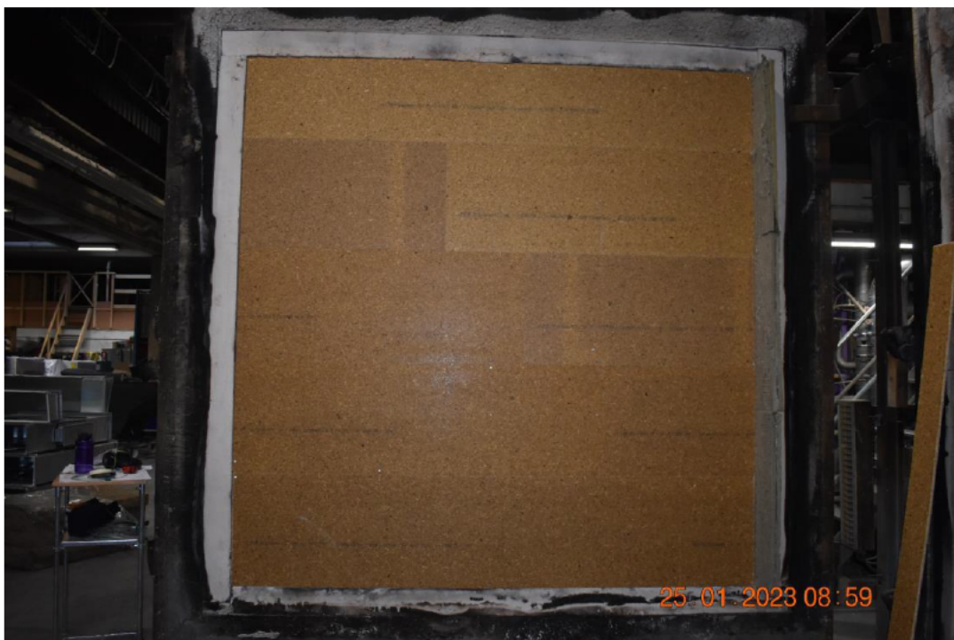
Photo No. 4 Test specimen seen from exposed side during mounting
