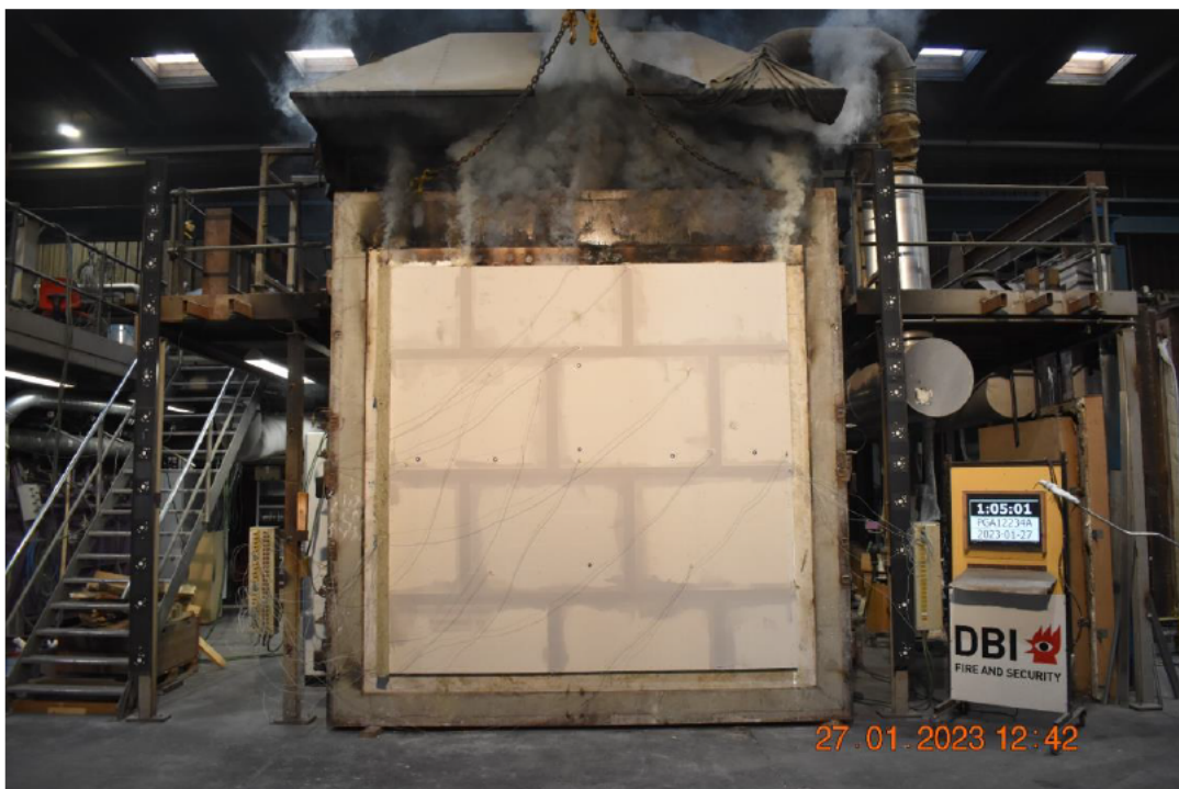
Photo No. 14 Test specimen seen from unexposed side 65 minutes into the test
