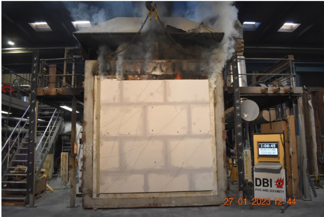
Photo No. 15 Test specimen seen from unexposed side 66 minutes into the test
