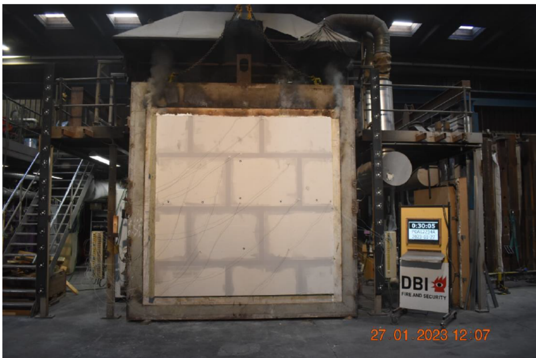
Photo No. 12 Test specimen seen from unexposed side 30 minutes into the test
