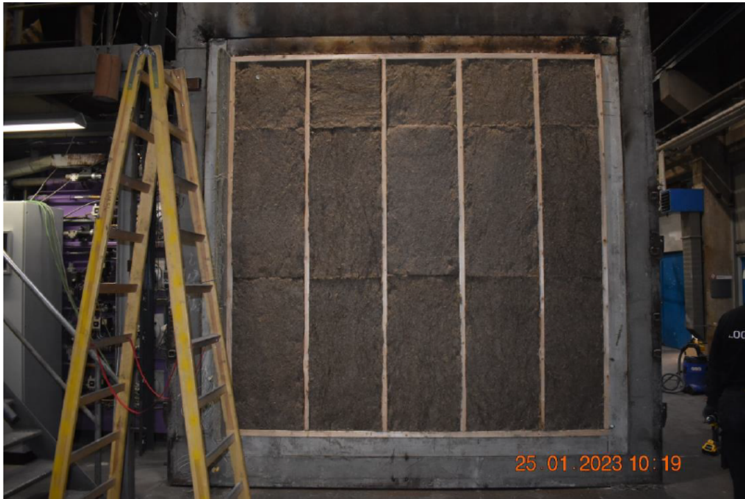
Photo No. 7 Test specimen seen from unexposed side during mounting
