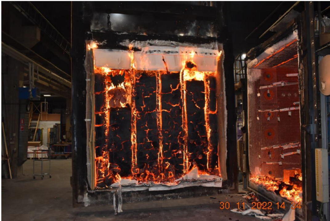
Photo No. 19 Test specimen seen from exposed side after the test
