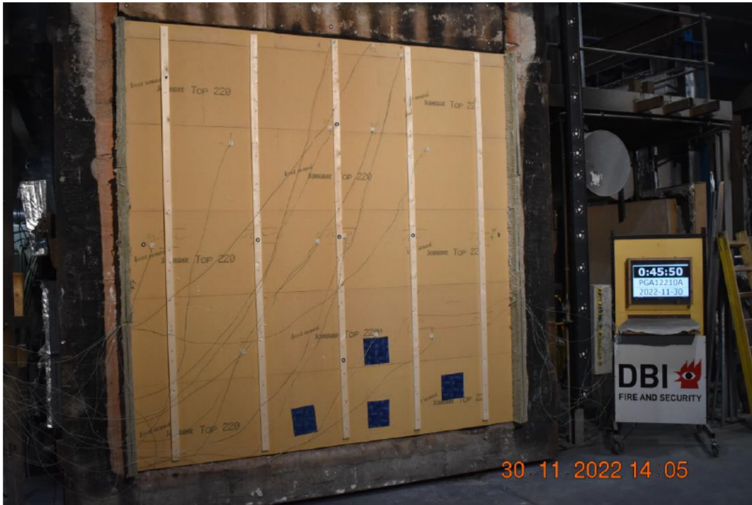
Photo No. 13 Test specimen seen from unexposed side 45 minutes into the test
