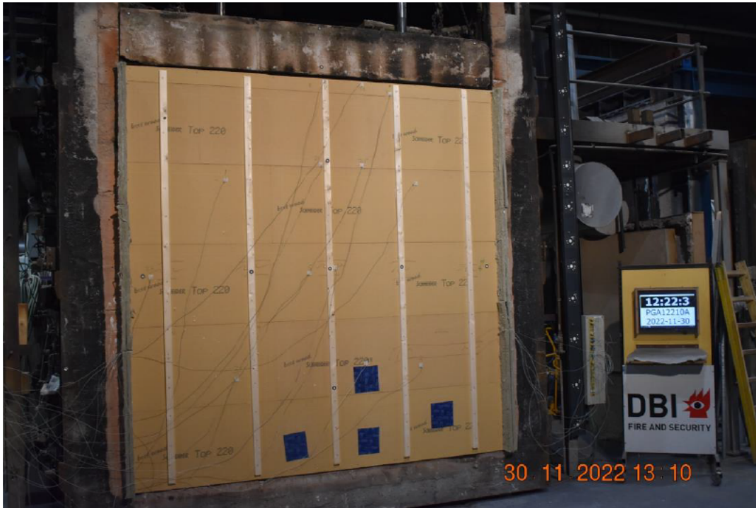
Photo No. 9 Test specimen seen from unexposed side before test start
