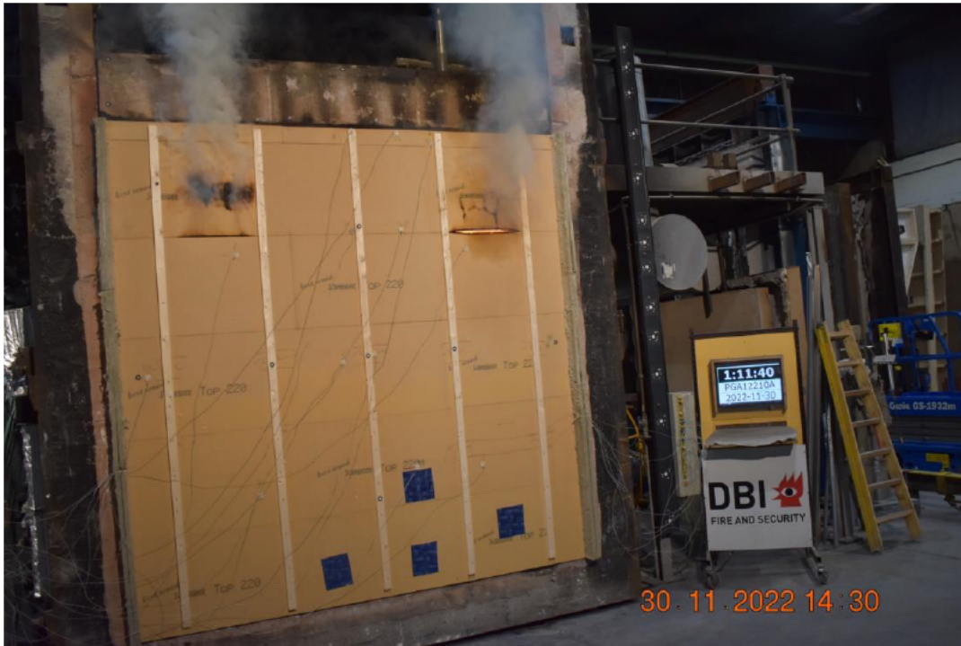
Photo No. 17 Test specimen seen from unexposed side 71 minutes into the test
