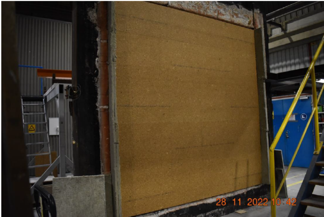
Photo No. 3 Chipboard mounted on exposed side
