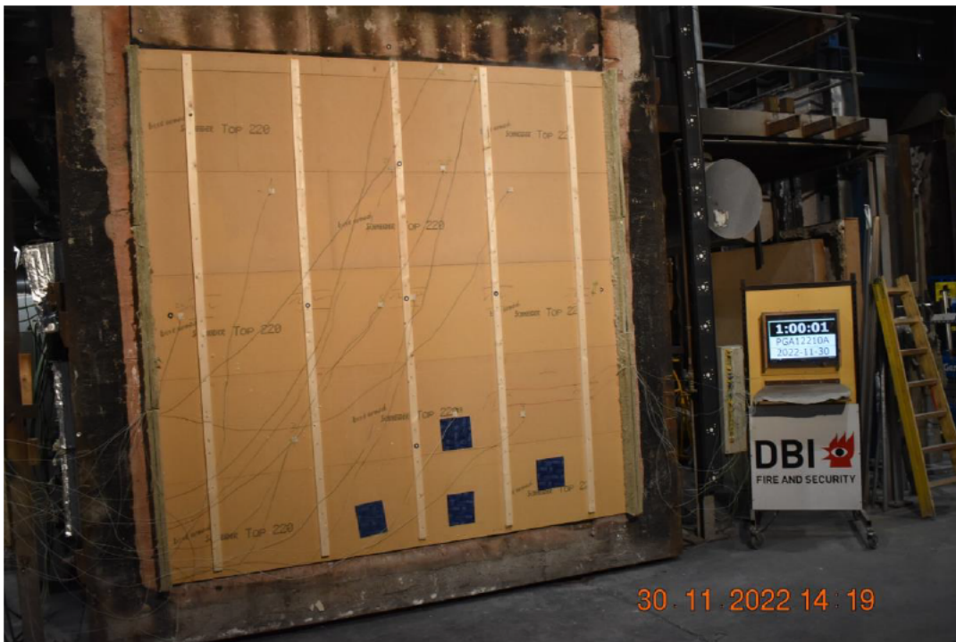
Photo No. 14 Test specimen seen from unexposed side 60 minutes into the test
