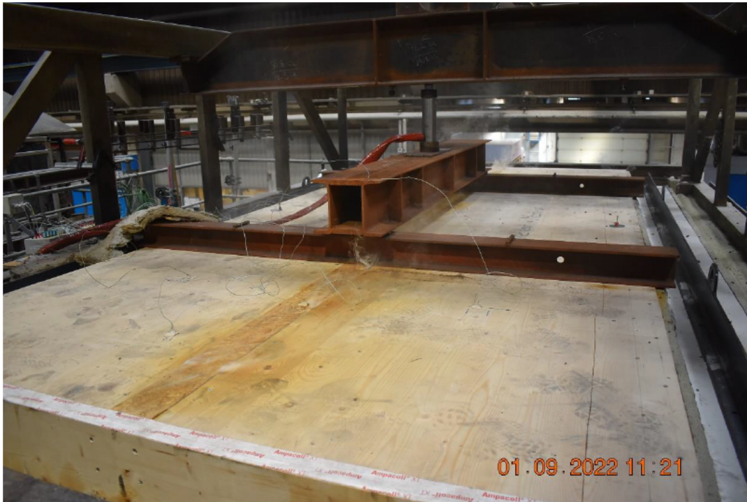
Photo No. 27 Test specimen after 74 minutes of testing
