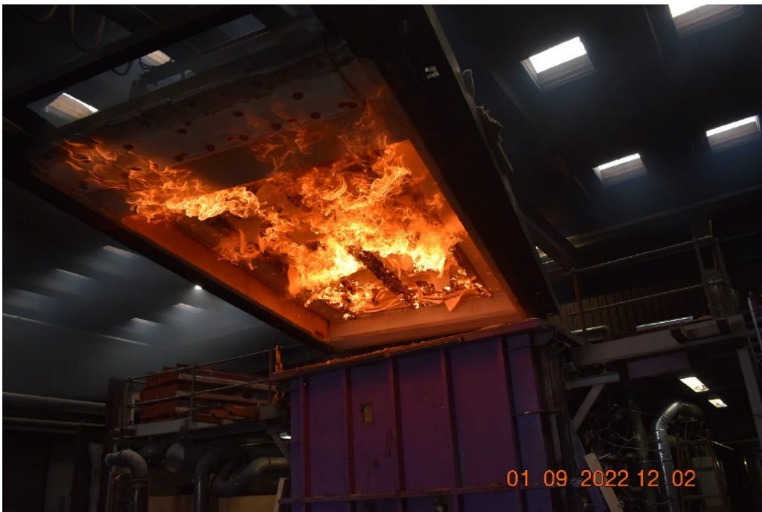
Photo No. 32 Exposed side when the test specimen is removed from the furnace, five minutes after test is stopped
