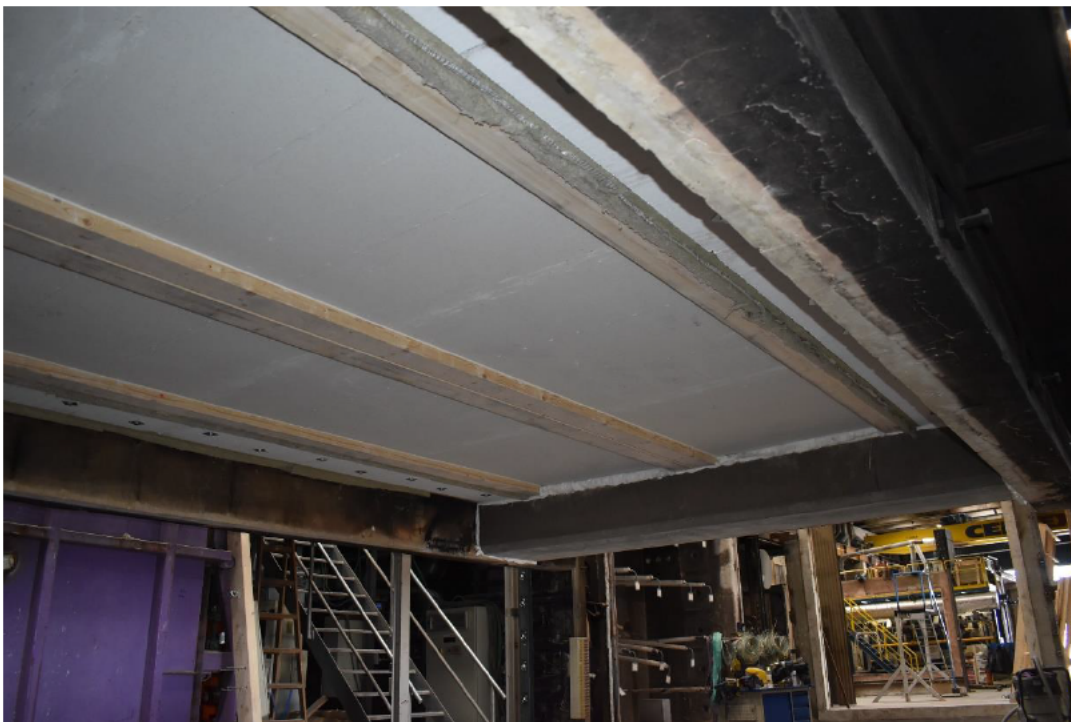
Photo No. 20 Test specimen mounted in frame seen from exposed side
