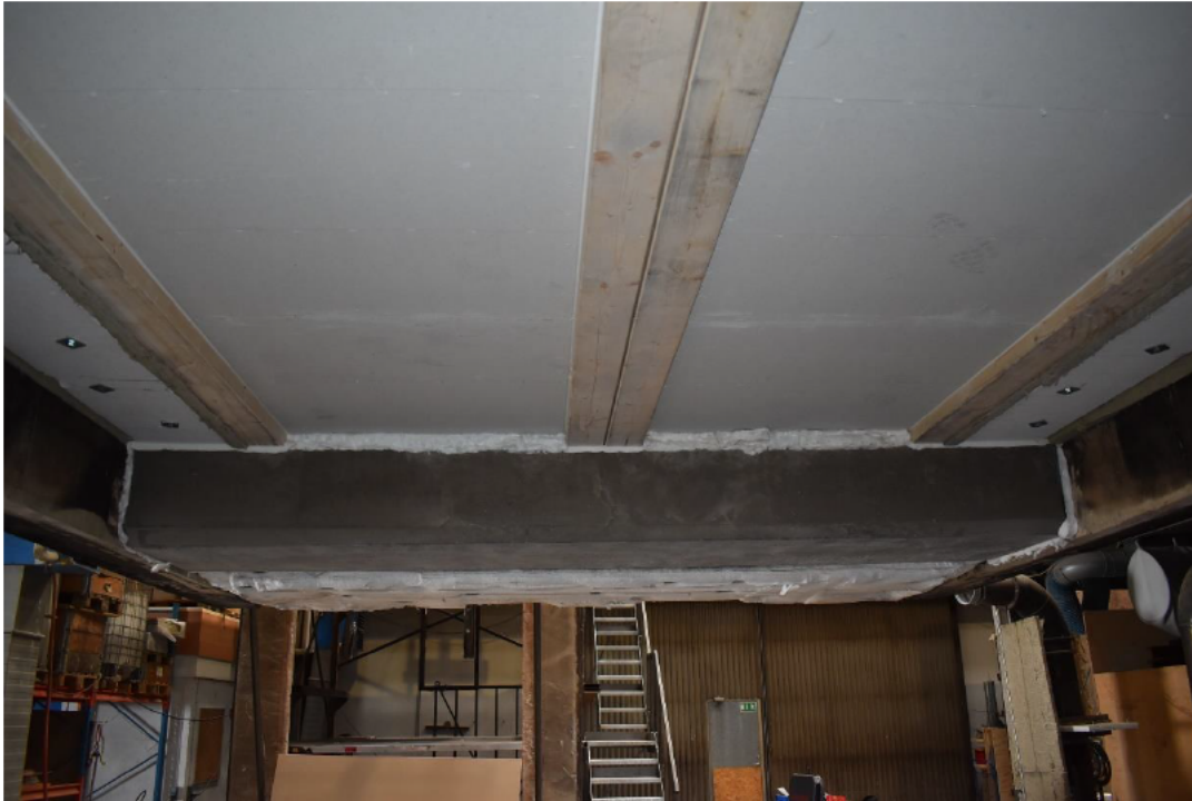
Photo No. 21 Test specimen mounted in frame seen from exposed side
