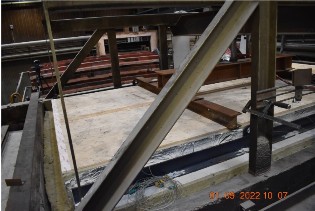
Photo No. 23 Unexposed side when the test starts
