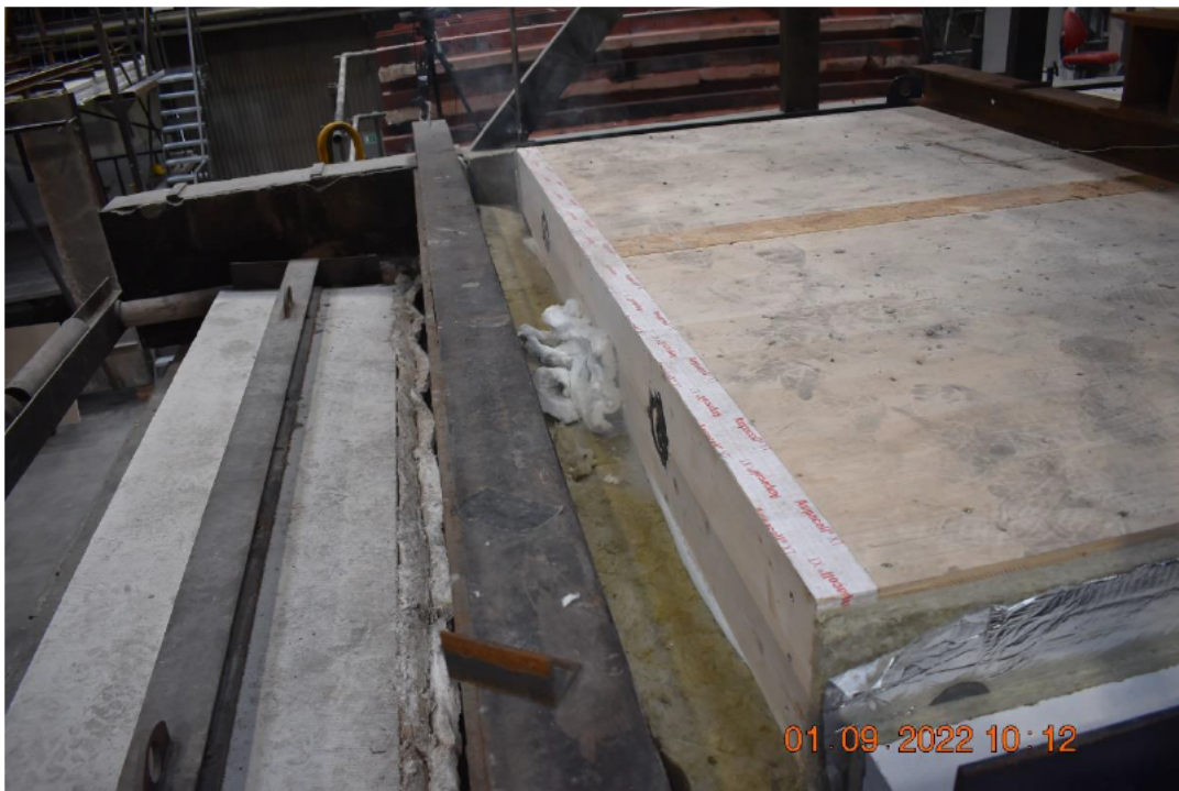
Photo No. 24 Gaps on short edges of test specimen is insulated during the test
