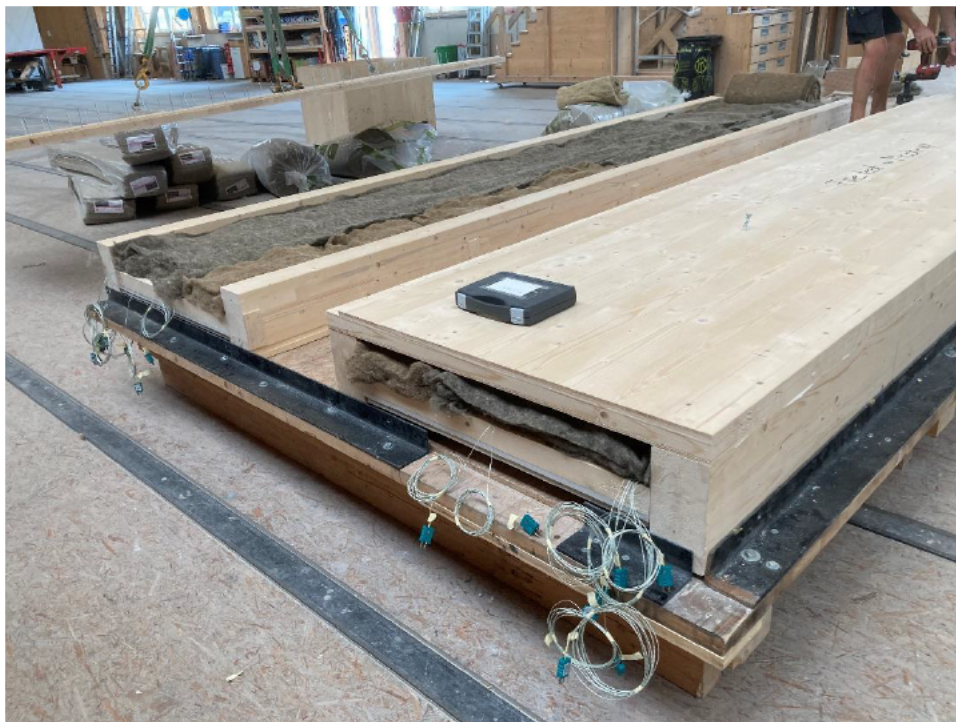
Photo No. 6 The first element glued and screwed
