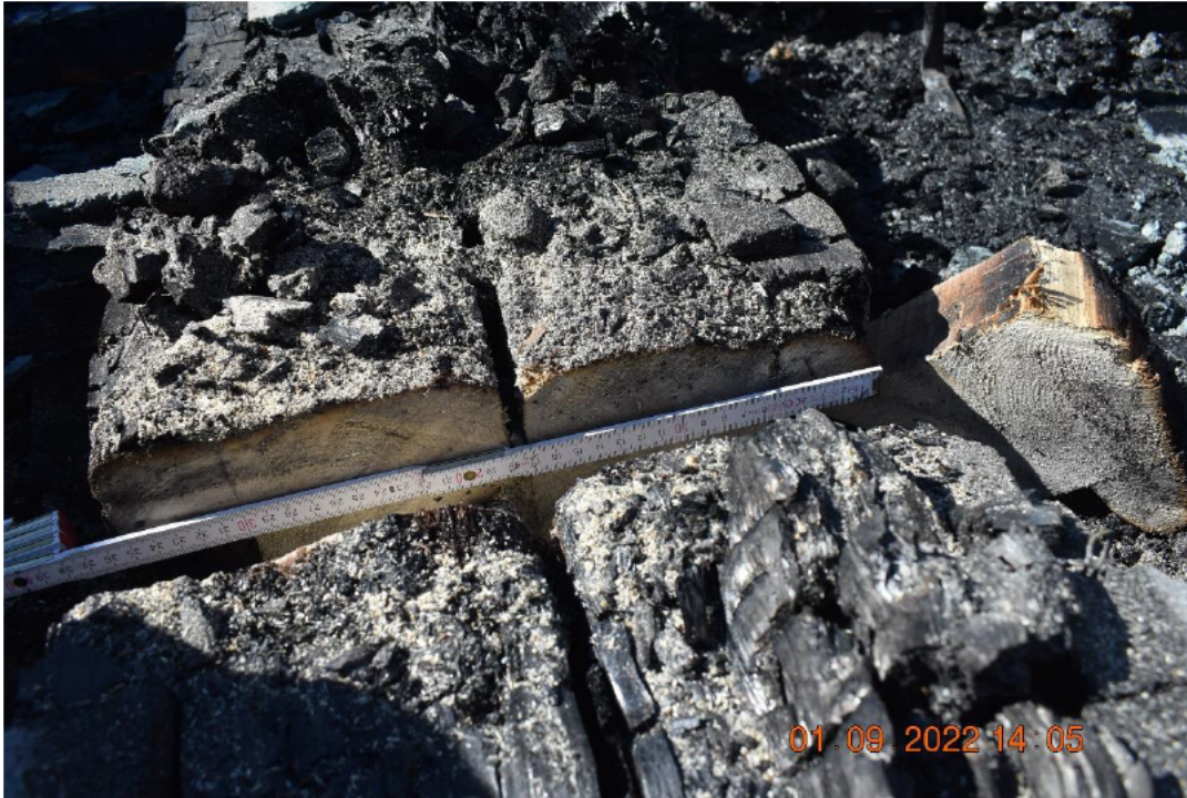
Photo No. 35 Charring of centre timber beams after test
