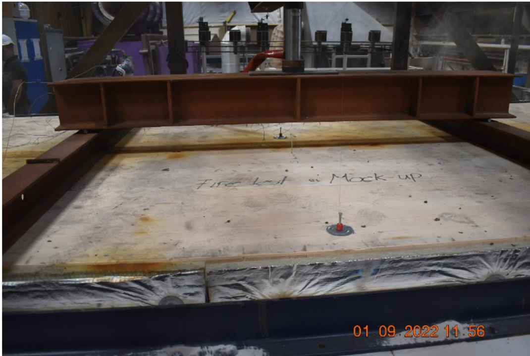
Photo No. 29 Test specimen after 109 minutes of testing
